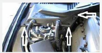
Remove the (3) screw pins that hold the battery cover to the body lift up the battery cover and disconnect the negative battery terminal using a 10mm socket.
