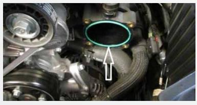
Be sure to clean the O-Ring of any oils or dirt before installing the BBK throttle body.
