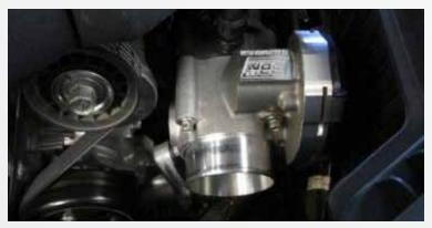
Install the BBK 65mm throttle body using the stock hardware and snug the bolts down.
