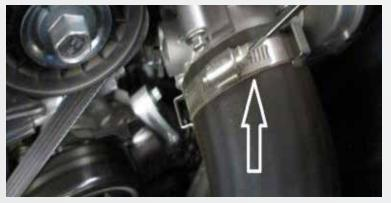
Loosen the clamp on the air inlet tube that connects to the throttle body using a flat head screwdriver or 7mm socket. Remove the air inlet hose by pulling it towards the front of the vehicle and slightly wiggling it side to side.
